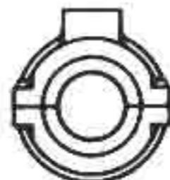
BEARING in HANGER
